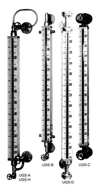
Three-color interface gauge is based on differential specific gravity of two liquids. Glass float with special plating cover floats on interface. The float is very striking, at same time, liquid level is indicated with red gas and green liquid.
